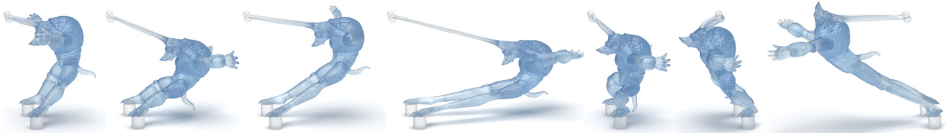
Fig. 9. Dragging Armadillo. To objectively examine the convergence of our method, we simulate an elastic Armadillo under large deformations in a collision-free setting using projected Newton (multi-core CPU, MKL), gradient descent (GPU, CUDA), and our method (GPU, CUDA). The model consists of 500K elements and 300K DOFs. Because collisions are ignored, the comparison does not include the warm-start step or local/regular CCD.
