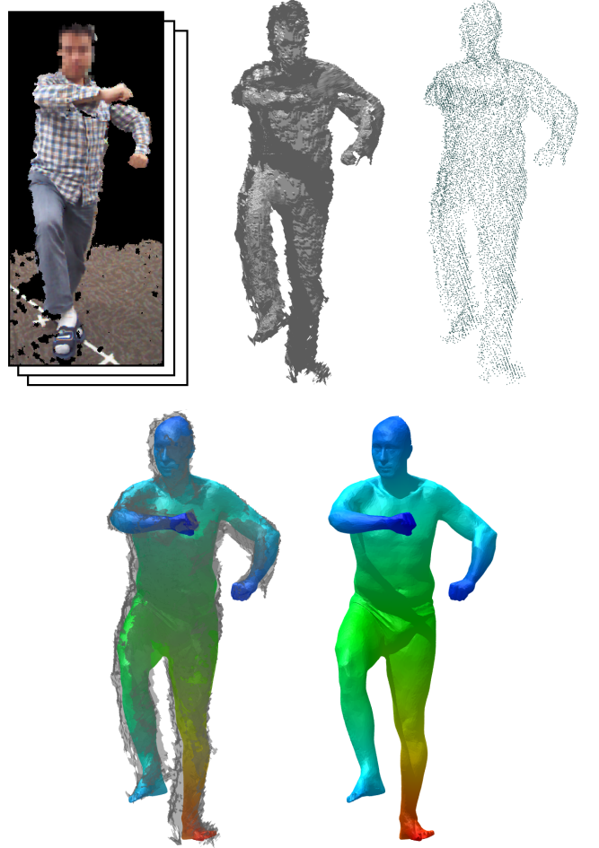
Figure 6: Process of posing by depth camera data. Top row, from left to right: pose is captured by three cameras from different views, captured pose in 3D, captured pose is down sampled to about 20K points for deformation. Bottom row: posed template overlapped with captured pose, posed template.
