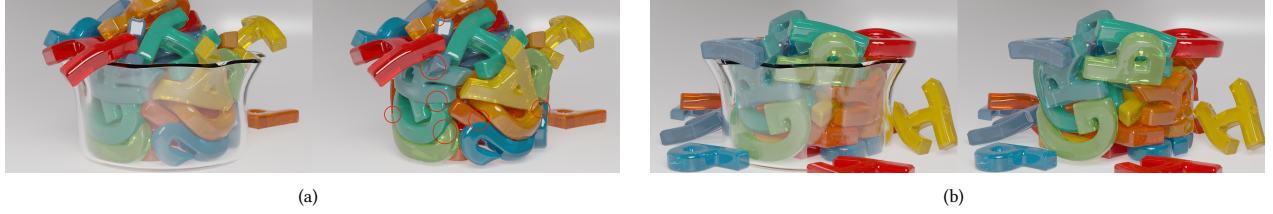
Fig. 7. The data synchronization strategy greatly impacts simulation accuracy. (a) Averaging positions can result in penetrations, while (b) averaging displacements ensures correct collision handling.
