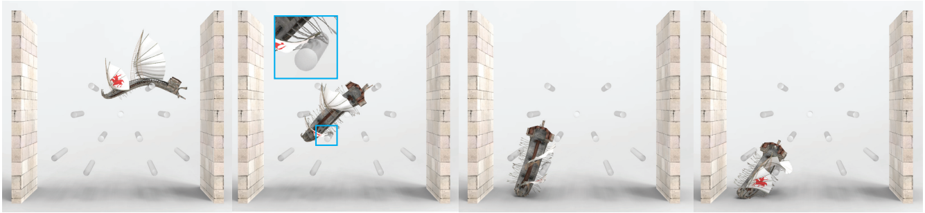
Fig. 1. Our framework couples spatial model reduction and collision detection via medial axis transform, a high-fidelity and compact volumetric shape representation. This representation (known as the topological skeleton) does not only provide us an expressive subspace, but also serves as a tight volume enclosure to facilitate the collision detection and handling. In this figure, the barbarian ship has 482k elements and 236k triangles. Following a semi-reduced projective dynamics formulation, this model is reduced to a 2, 526-dimension subspace with 482k constraints. The animation runs at \sim 15 FPS with all the collisions and self-collisions resolved and rich local details preserved.
