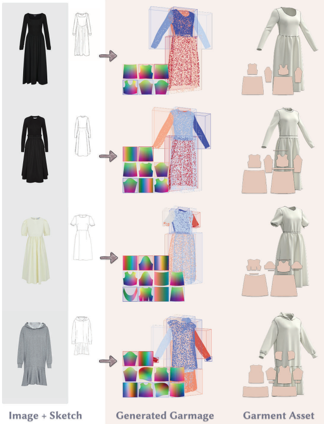
Fig. 16. Image-guided Garmage generation results. We transfer the image to line-art sketches (top right corner) with a LoRA finetuned FLUX model, then use the transferred sketch as input condition to control the generation of Garmage. The generated Garmages and simulated garment assets are demonstrated on the right side.
