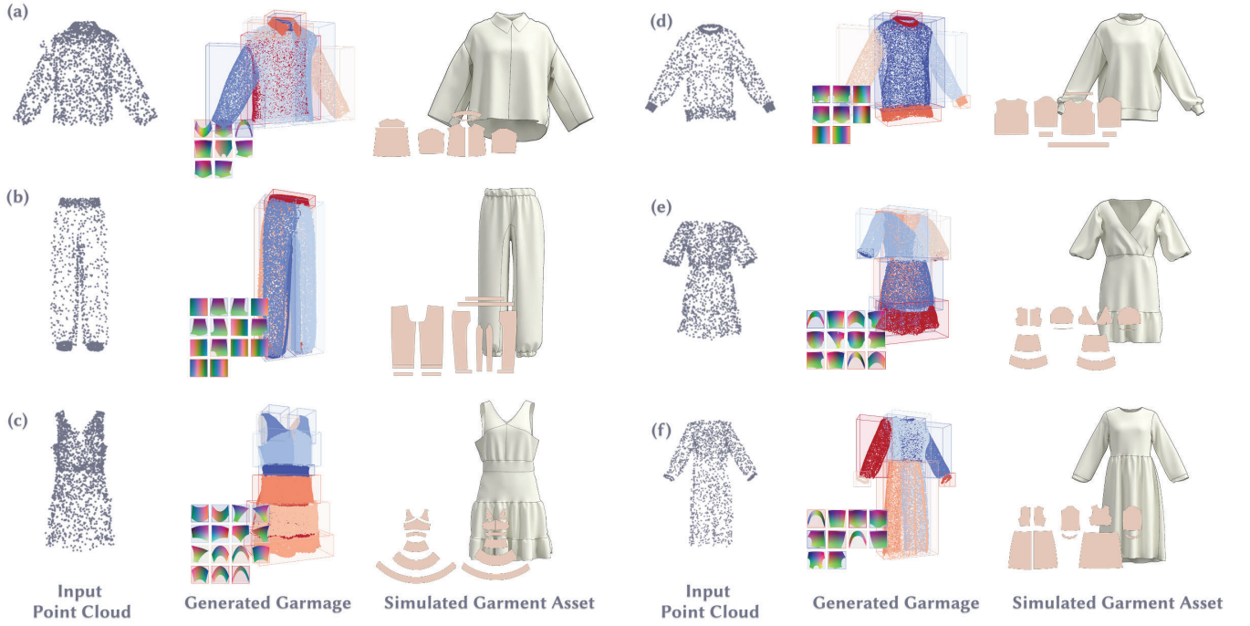
Fig. 18. Point-cloud-conditioned garment synthesis with GarmageNet . Each row (a–f) shows: (left) an unstructured, sparse point cloud captured from a draped garment; (center) the generated Garmage representation—consisting of per-panel geometry images (colored) and inferred panel contours (outlined); and (right) the final simulation-ready 3D garment asset, obtained by vectorizing the extracted sewing patterns, recovering vertex-wise stitches, and applying physics-based draping. These results demonstrate GarmageNet’s ability to transform noisy, incomplete point clouds into fully structured sewing patterns and high-fidelity draped garments. We note, however, that the network may be leveraging the non-uniform sampling density of the input point clouds—implicitly revealing panel structure—to achieve these reconstructions.
