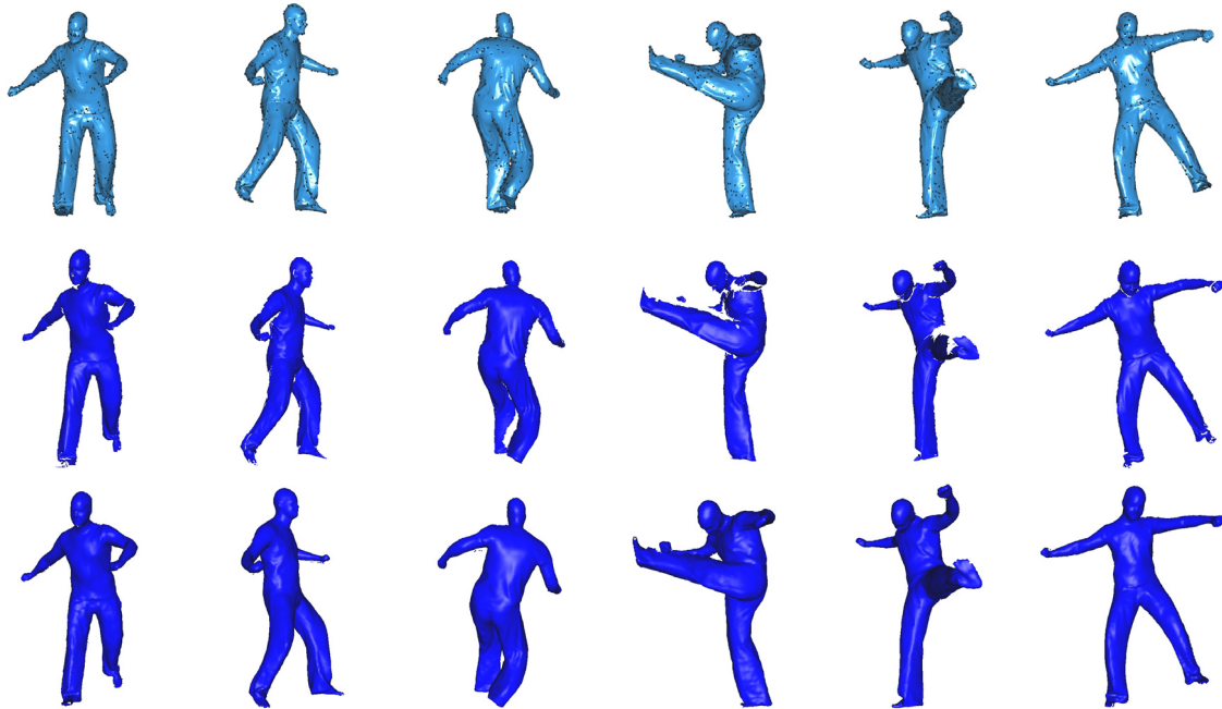
Figure 5. Six frames (frame 1, 10, 17, 24, 29 and 35 out of all 38 frames) are shown in this figure. 1 st row shows the rendered models. The black dots indicate the tracked features. 2 nd row is the partial meshes constructed from depth maps. The 3 rd row shows the reconstructed 3D models by our algorithm.
