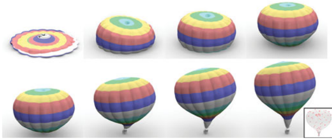
Fig. 11. Use reduced IFE simulation to imitate the inflation of a hot-air balloon. In this example, we simply use Cubature points as restorative elements. Three domains are defined.
