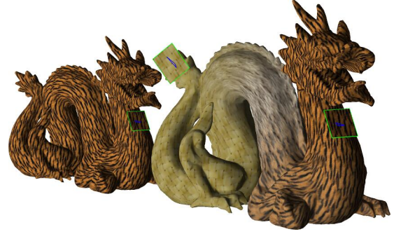
Figure 9: A new material constraint is added to the dragon's tail (right) and is interpolated across the surface. The clamping ensures that the material m remains in a valid range on the dragon's head.
