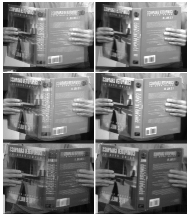
Figure 13: Synthesized results of the book sequence. Left: traditional LFR with unsynchronized frames. Right: Space-time LFR.
