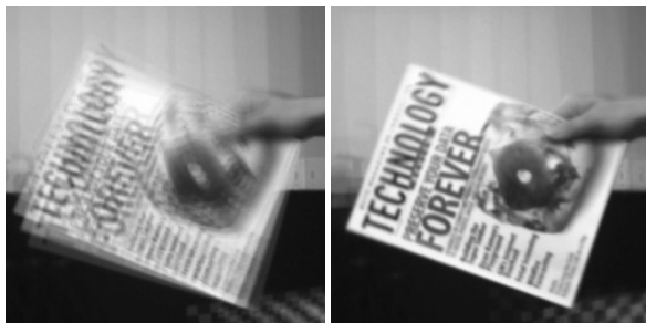
Figure 12: Synthesized results using a constant blending weight (i.e., pixels from all frames are averaged together). Left: traditional LFR with unsynchronized frames. Right: Space-time LFR.
