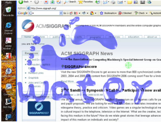
Figure 6: INTERACTIVE: Fluid control by external accelerations due to the motion of a user's cursor.
