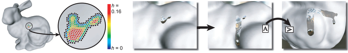
Figure 3: BUNNY: The left picture illustrates spatial discretization and the cell connectivity on the bunny model. Colored cells are water cells and black cells are boundary cells. The right picture shows a water drop changes its path after the bunny model was rotated 90°.
