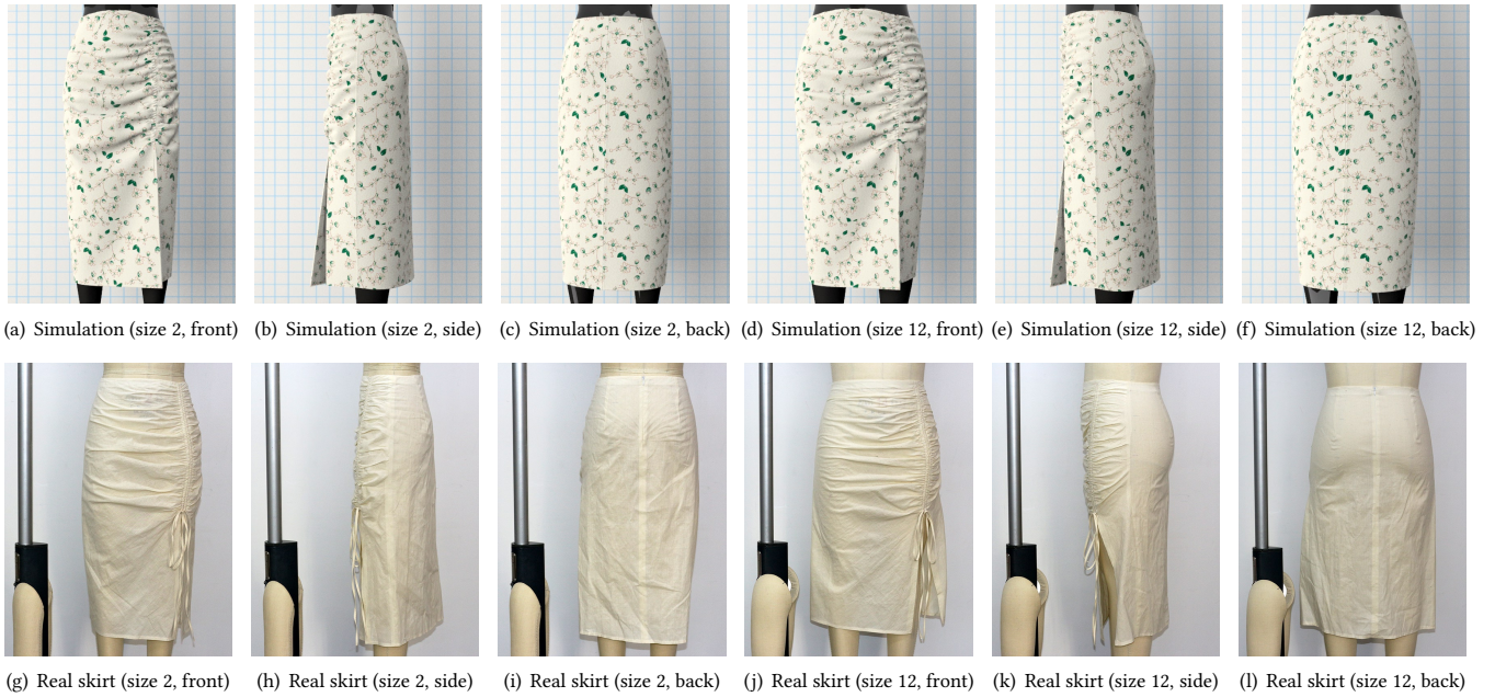
Fig. 11. The automatic grading results of a Carmen skirt example. Our system can flexibly handle complex patterns designed to create garments with shirring, as demonstrated on the left side of this Carmen skirt.
